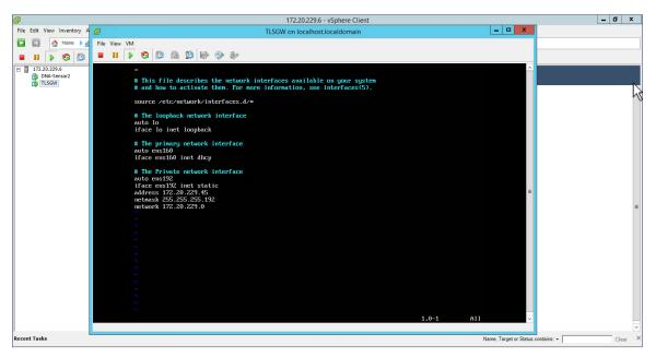
**Step 7** To restart the network service, go to /etc/init.d and type ./networking restart. Now, do a ifconfig and you should see both the Public interface IP address and Private interface IP address. Ping both Public and Private IP address to verify connectivity.
