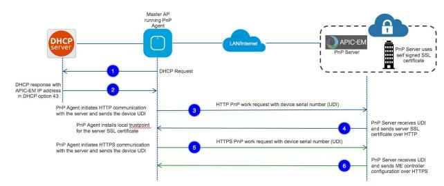
Option 43 points to APIC-EM controller IP address. To configure DHCP scope with Option 43, it is important follow the format as shown below. In the example below, 192.168.1.123 is the IP address of APIC-EM controller
