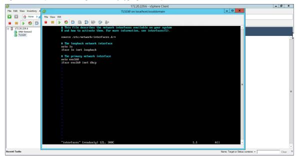
Note: *ens160* is Public network interface and is configured for DHCP by default. If you want to statically configure the IP address of Public network interface, replace the *ens160* setting with the following as shown below in the example.
