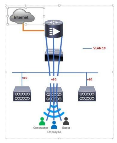
On Mobility Express, management traffic is untagged. If Access Points and WLANs are all on different VLANs, Mobility Express capable Access Points will connect to a trunk port on the switch and traffic for individual WLANs will be switched locally on individual VLANs. Shown below is a deployment with Access Points and WLANs on different VLANs.
