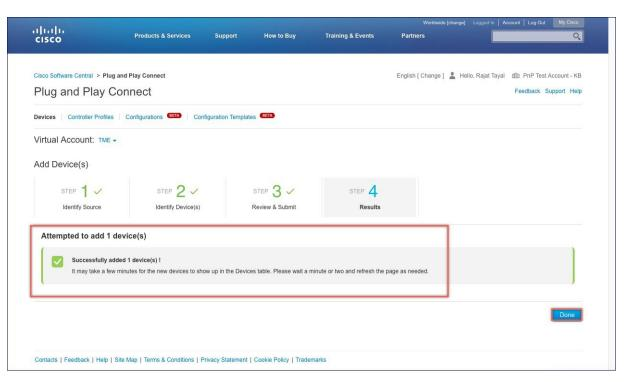
**Step 7** Verify that the Device has been added and the status is Pending (Redirection).
