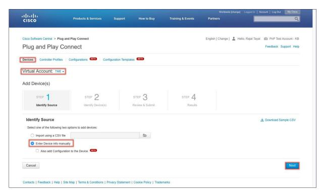
Step 5 Click on Identify Device button. The Identify Device window will pop up. Enter Serial Number, select Base PID, and Controller Profile(created earlier). Click on the Save button followed by Next button.
