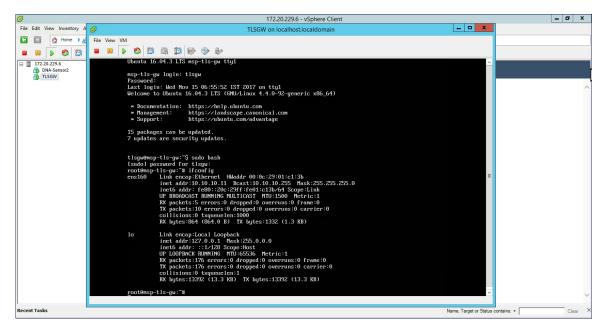
**Note** *ens160* corresponds to the Public network interface and in the above example it has got the IP of *10.10.10.11* from the DHCP server. One can also statically assign the IP address which will be shown the steps ahead. Also, there is no interface for the Private network in the *ifconfig* output above. We can also manually configure this and is shown in the steps ahead.
