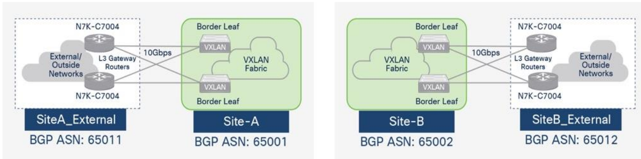
Figure 16. MP-BGP External Connectivity in Site-A and Site-B
