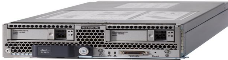
Figure 17 Cisco UCS B200 M5 Blade Server
