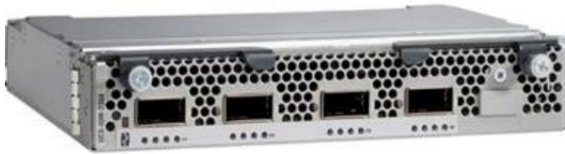
Figure 21 Cisco UCS 2304XP Fabric Extender
