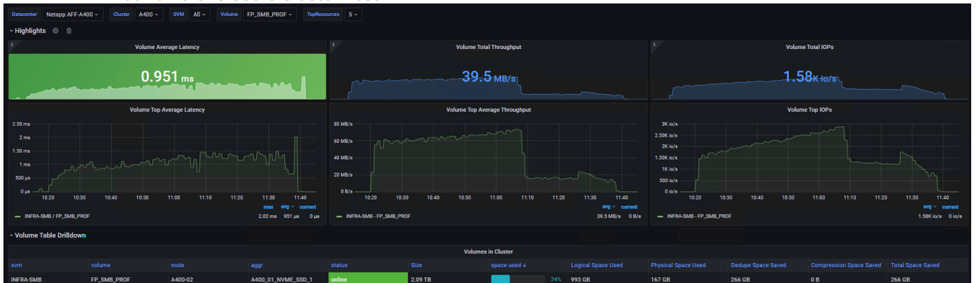
Figure 126. Volume Average Latency, Volume Total Throughput and Volume Total IOPS AFF A400 SMB Share for 1700 Full Clone Users Cluster Test
