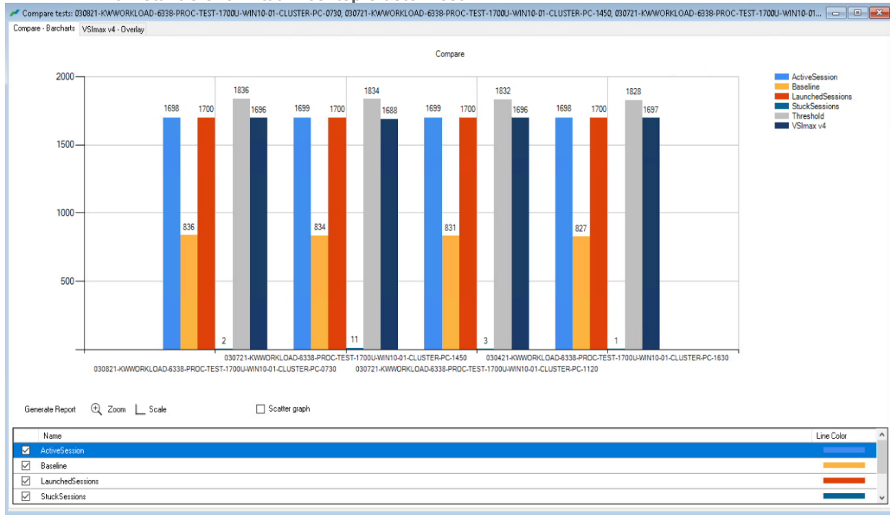
Figure 111. Login VSI End User Experience Comparison for 4 repeat tests for FullScale 1700 single session Win 10 Instant Clone Virtual Desktop Cluster Test
