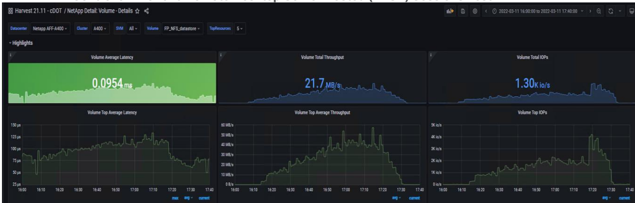
Figure 70. Volume Average latency, Volume Total Throughput and Volume Total IOPS from AFF A400 Storage Controller 2 for 325 Remote Desktop Server Hosted (RDSH) Sessions Test
