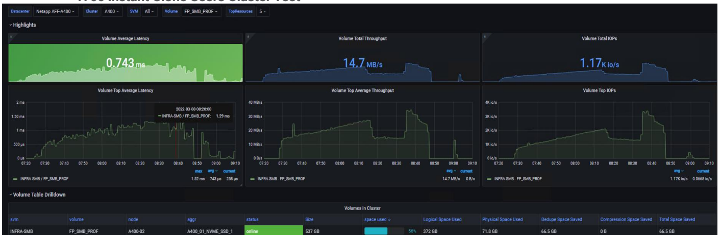
Figure 117. Volume Average Latency, Volume Total Throughput and Volume Total IOPS AFF A400 SMB share for 1700 Instant Clone Users Cluster Test
