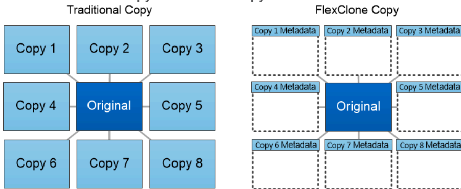
Figure 17. Traditional Copy vs FlexClone Copy
