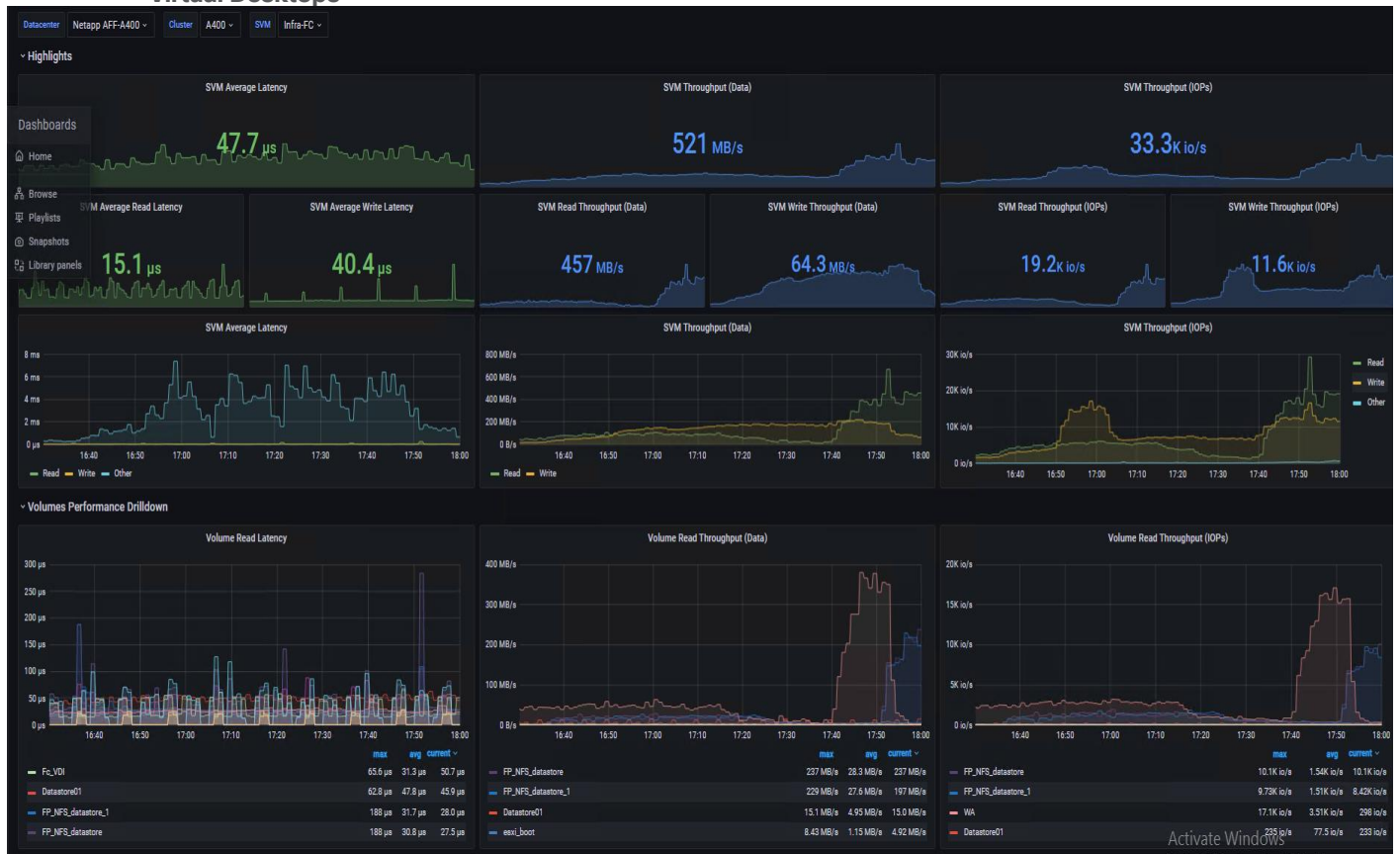
Figure 84. SVM Average latency, SVM Total Thruput and SVM Total IOPS from AFF A400 Storage for 245 Win 10 Virtual Desktops
