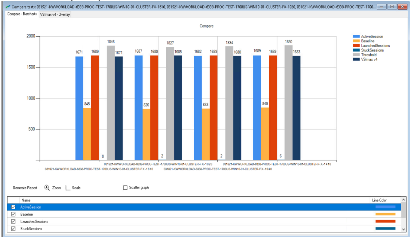
Figure 120. Login VSI End User Experience for 4 Repeat Tests: Full Scale test 1700 Full Clone Win10 Virtual Desktops Comparison
