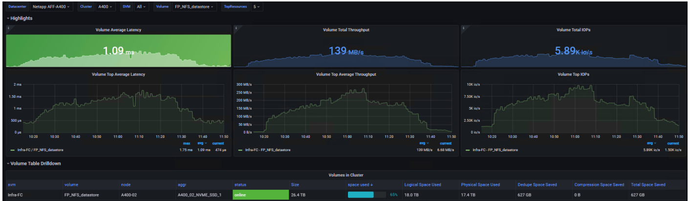
Figure 125. Volume Average Latency, Volume Total Throughput and Volume Total IOPS AFF A400 Controller 2 for 1700 Full Clone Users Cluster Test
