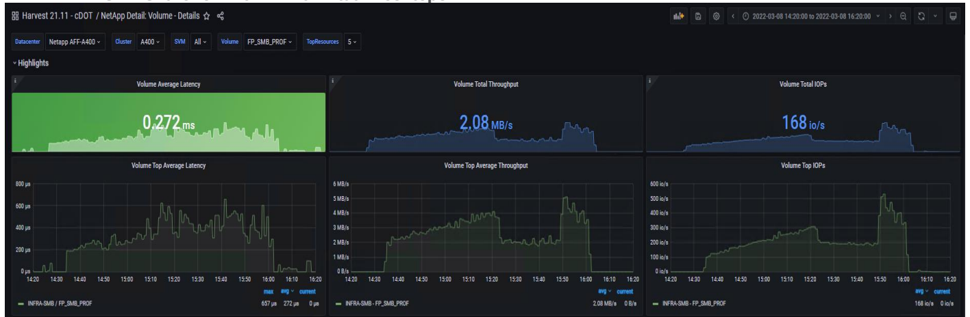
Figure 83. Volume Average latency, Volume Total Throughput and Volume Total IOPS from AFF A400 Storage for SMB Share for 245 Win 10 Virtual Desktops
