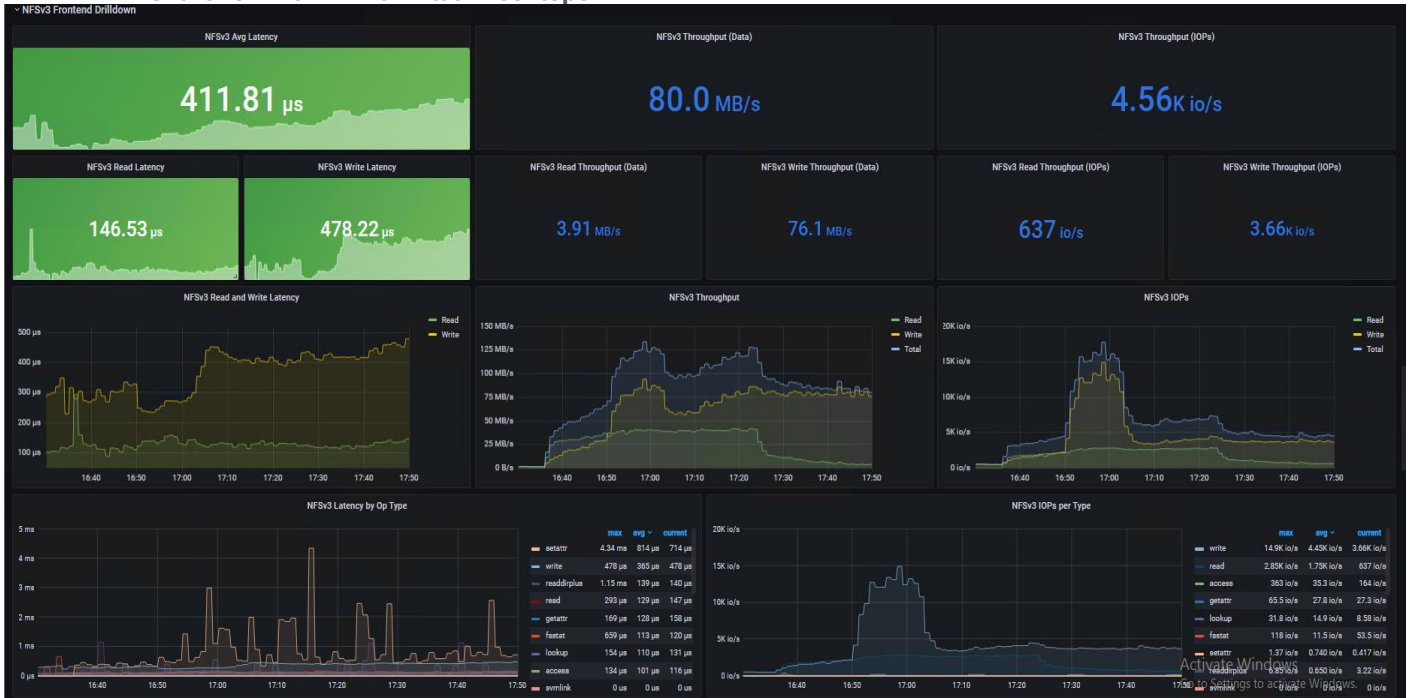
Figure 87. NFSv3 Avg Latency, NFSv3 Throughput and NFSv3 Throughput IOPS from AFF A400 Storage for SMB Share for 245 Win 10 Virtual Desktops
