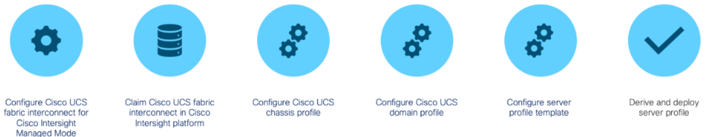
Figure 5. Configuration Steps for Cisco Intersight Managed Mode
