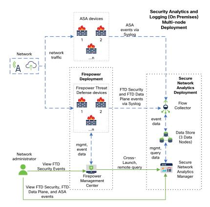
In this deployment, the Firepower Threat Defense and ASA devices send Firewall events to the Flow Collector. The Flow Collector sends the events to the Data Store (3 Data Nodes) for storage. From the Firepower Management Center UI, users can cross-launch to the Manager to view more information about the stored events. They can also query remotely the events from the Firepower Management Center.
