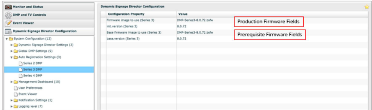
Figure 3 Firmware Image and Version Properties Required to Provision the CV-UHD and CV-HD
