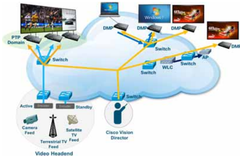
Figure 5 IP Multicast Overview
