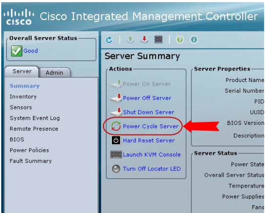
Figure 8 Power Cycle Server From the CIMC Console
