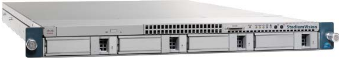
Figure 1 Front Panel of a Cisco StadiumVision Director Platform 2 Server
