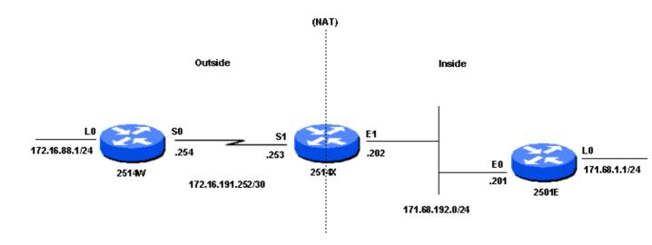
When ping is sourced from the Router 2514W Loopback0 interface (172.16.88.1) to the Router 2501E Loopback0 interface (171.68.1.1), this occurs:
