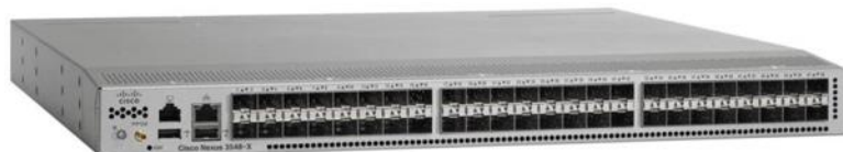
Figure 7. Cisco Nexus 3548-XL and 3524-XL Switch
