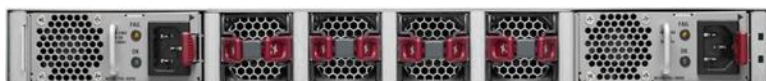
Figure 9. Cisco Nexus 3548-XL and 3524-XL with red handles indicating port-side intake airflow
