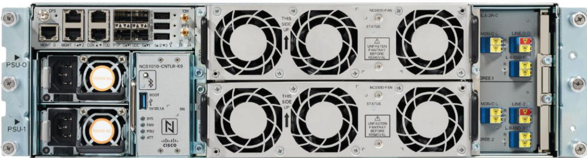
Figure 13. NCS 1010 ILA-2R-C card with Raman amplification on both directions
