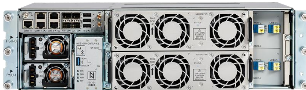
Figure 15. NCS 1010 ILA-C amplifier card without any Raman amplification for C-Band
