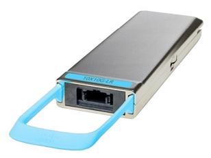
**Figure 5.** Cisco CPAK-10X10G-LR Module
