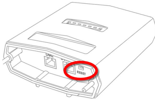
Figure 8. Cisco FM3200 Base (Hardware RESET button port)
