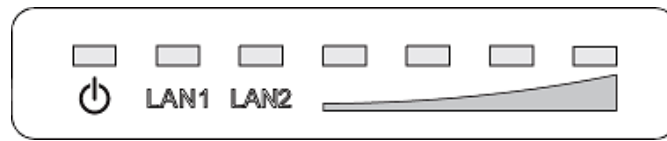
Figure 6. Status and link/boot LEDs
