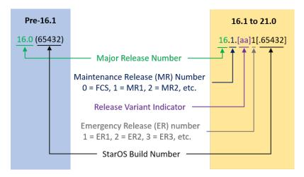
The Version Build Number for releases 21.1 and later include a major and emergency release number, for example, "21.1.1".
