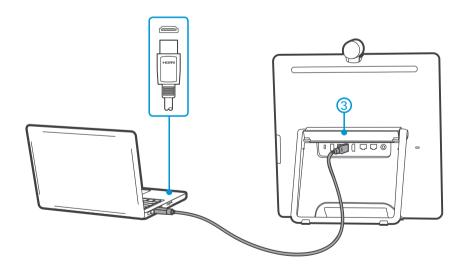
The DX70 can be connected to an external monitor via the HDMI out port.
