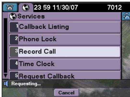
Figure 8: Cisco IP Phone Services Key Showing Record Call Option
