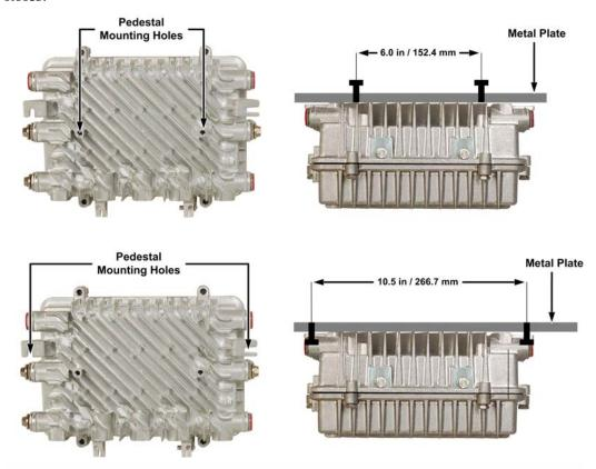
4 Using a ½-inch torque wrench, tighten the Pedestal clamp bolts from 6.8 Nm to 9.0 Nm.
