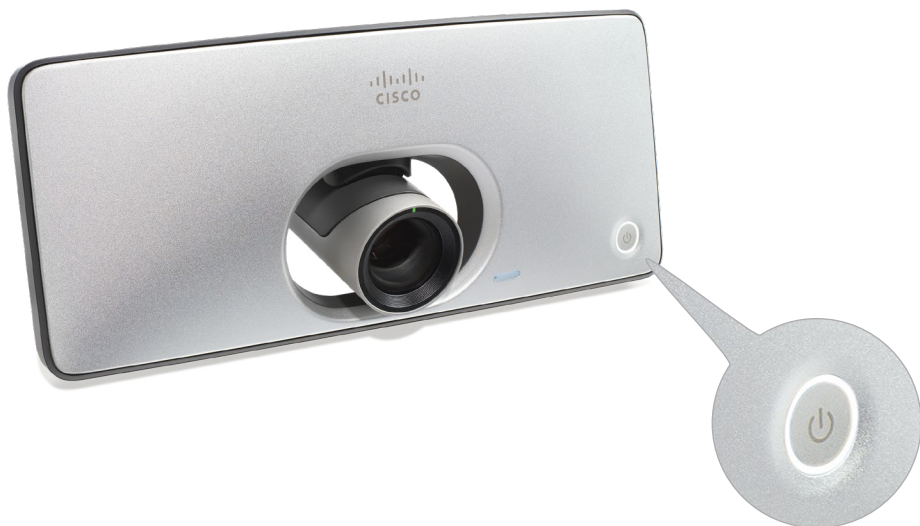
Power button with LEDs encircling the button
