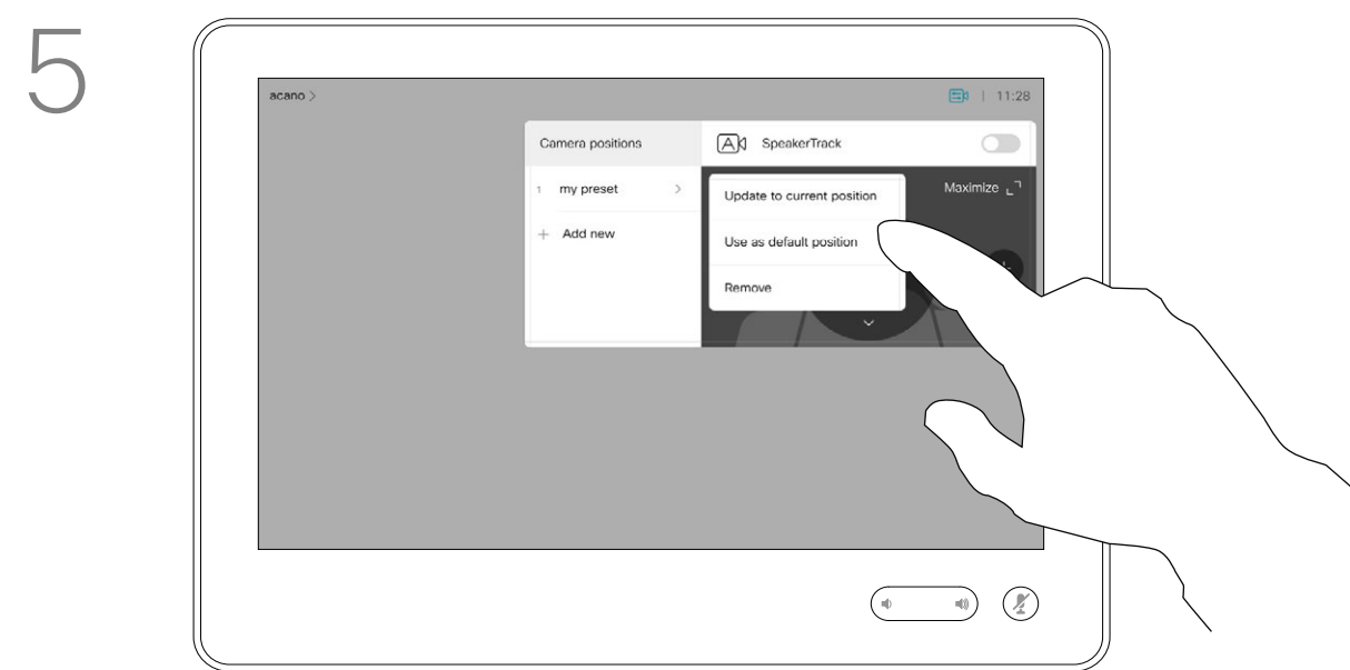
Tap Update to current position to put your changes into effect. To delete an existing preset tap Remove .
