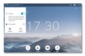
You can set restrictions to users' access to the settings menu. This can be done on the web interface. Go to *Setup* > *Configuration* > *User Interface* and set *User Preferences* to *Off.* With this restriction, only *System Information, Call Status, Diagnostics* and *Restart* are available for the users.
