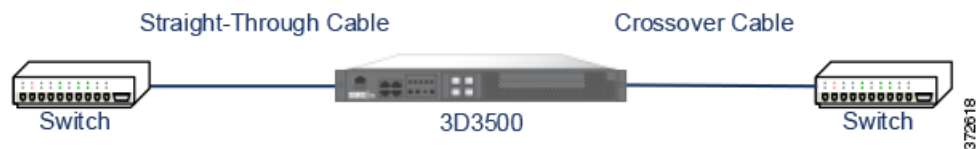
Figure 2-1 Straight-Through Bypass Connection Cabling
