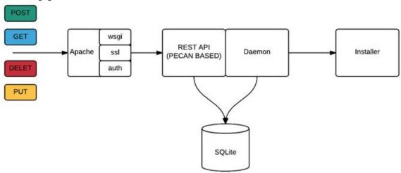
The Cisco VIM REST API security is provided by the Secure Sockets Layer (SSL) on the Apache web server. The *mod\_wsgi* running on the Rest API server calls the Pecan-based web application. The Pecan REST API server requires a username and password to authorize the REST API server requests.
