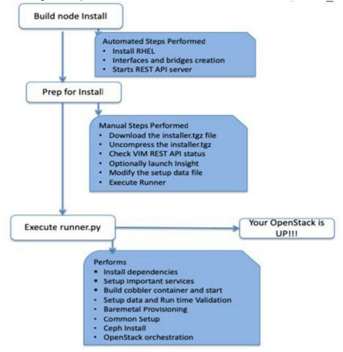
If you have Cisco Unified Management (UM), complete only part of the Cisco VIM installation procedure and proceed to the Installing UM with Internet Access procedure to complete the configuration and setup of Cisco VIM. If you do not have Cisco VIM UM, configure Cisco VIM by editing the setup\_data. yaml file as described in the Cisco VIM installation.
