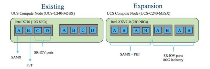
For computes with 25G NICs, the lower two NIC slots are used for control and data plane. Hence, care must be taken in placing the NICs across the NUMA node. In an UCS 240 M5 node, use slot 1 for the first 25G NIC, and slot 4, 5, and 6 for next 3 25G NIC cards to yield a balanced virtual network across NUMA nodes. However, SRIOV is dedicated to a single NUMA.
