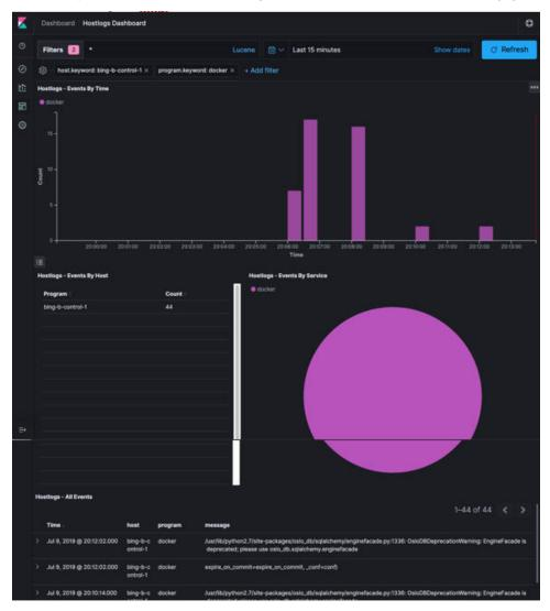
2. To know the log events in the Openstack for a given VM, enter the Lucene query (service: nova or service: neutron and message:<uuid>) in the **Fi Iters** field which is on top of the Dashboard. where <uuid> is obtained from Horizon website or by executing openstack nova list for the identifier
