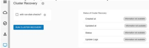
2. If you want to run disk checks, select with run-disk-checks? option, otherwise proceed with Step 3.
