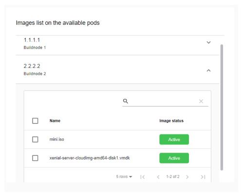
5. To delete a single/multiple image(s), select the image(s) to be deleted from the particular pod.
