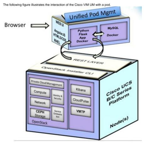
The architecture of the Cisco VIM UM is light-weight, hierarchical and scalable. It simplifies the management from the global UI. Each local site is autonomous with localized toolsets. The global UM UI provides ease of management with multi-site multi-pod capability for distributed NFV deployment at scale. Cisco VIM UM is designed to operate in HA as an option.
