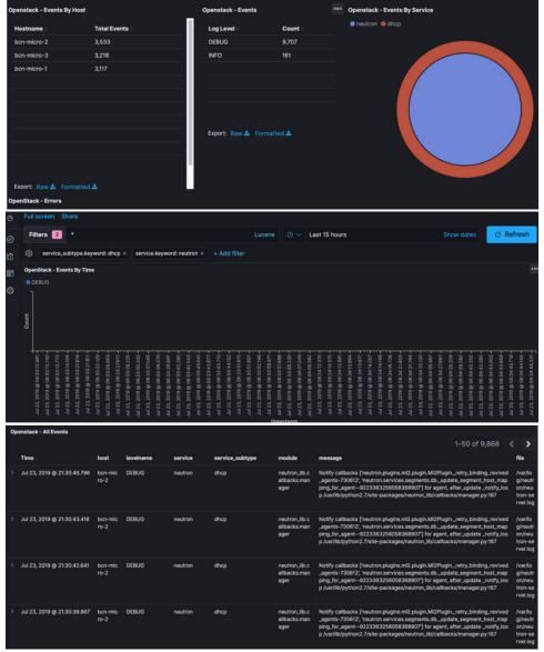
5. Without knowing the Lucene Syntax, you can set the filter criteria in the Search field using the Add a filter + option.
