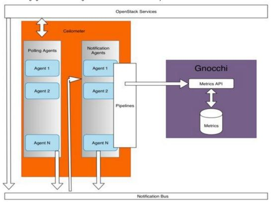
If ceilometer is enabled in setup\_data.yaml file, the Telemetry service in Cisco VIM collects the metrics within the OpenStack deployment.
