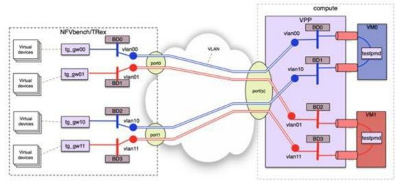
If VxLAN is enabled, it is possible to force the use of VxLAN using the -vxlan CLI option.
