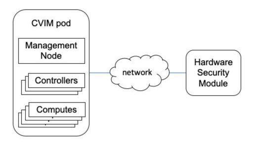
When Barbican is installed on a Cisco VIM pod, Cinder and Nova uses Barbican to store and retrieve volume encryption keys. Barbican is an optional service that can be included in the initial installation or added with a reconfigure operation. For details on how to enable Barbican see Enabling Barbican
