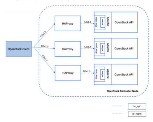
With TLS management network enabled, OpenStack endpoints are hosted over https. The required certificates are created during orchestration and then distributed to Cisco VIM nodes such as controllers and computes, so that OpenStack services communicate over a secure channel.
