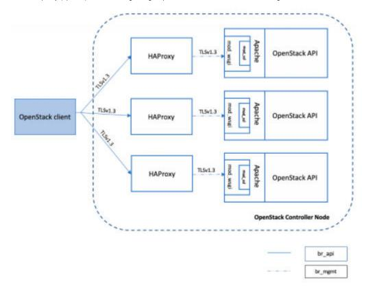
With TLS management network enabled, OpenStack endpoints are hosted over https. The required certificates are created during orchestration and then distributed to Cisco VIM nodes such as controllers and computes, so that OpenStack services communicate over a secure channel.
