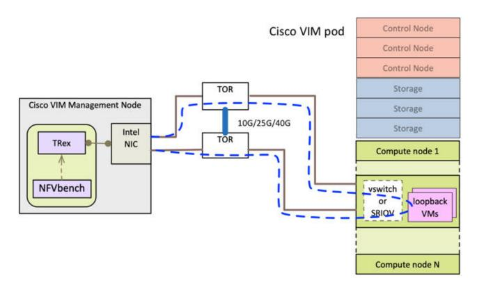
NFV bench runs on the management node inside a container along with the TRex open source software traffic generator. The traffic generator uses a dedicated Intel NIC to send and receive traffic to the ToRs.
