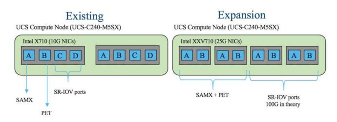
For computes with 25G NICs, the lower two NIC slots are used for control and data plane. Hence, care must be taken in placing the NICs across the NUMA node. In an UCS 240 M5 node, use slot 1 for the first 25G NIC, and slot 4, 5, and 6 for next 3 25G NIC cards to yield a balanced virtual network across NUMA nodes. However, SRIOV is dedicated to a single NUMA.
