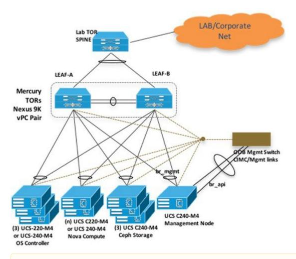
A Here, UCS 220 M4 is used as the control/compute, but UCS 240 M4 can also be used as control and compute nodes.
