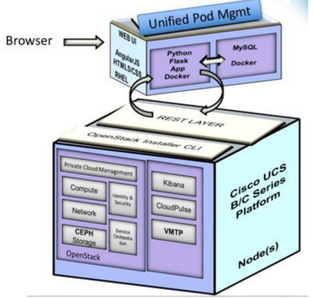
The architecture of the Cisco VIM UM is light-weight, hierarchical and scalable. It simplifies the management from the global UI. Each local site is autonomous with localized toolsets. The global UM UI provides ease of management with multi-site multi-pod capability for distributed NFV deployment at scale. Cisco VIM UM is designed to operate in HA as an option.
