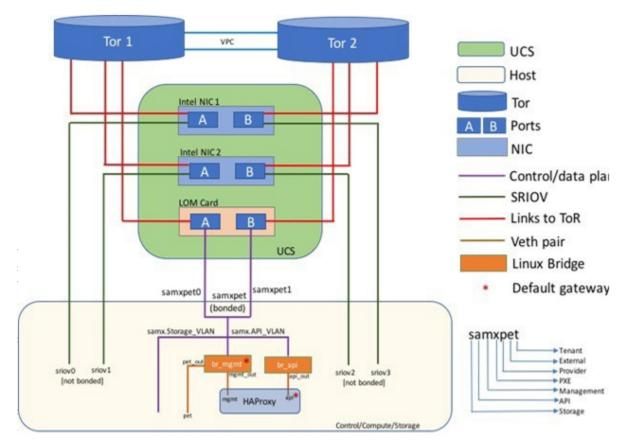
Cisco VIM 3.4.6 uses Dell PowerEdge 740 (with 2x1.2TB HDD) as compute with UCS M5 as control and ceph nodes in a full pod environment. In this configuration, four Intel XXV710 NIC cards are present in the compute with VPP/VLAN network. The cloud control and data plane are running on dedicated NIC cards, while the SRIOV is running on two additional NICs as depicted below:
