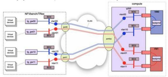
If VxLAN is enabled, it is possible to force the use of VxLAN using the –vxlan CLI option. The provision of custom configuration allows you to specify more VxLAN options such as specific VNIs to use. For more details, check the default configuration file.
