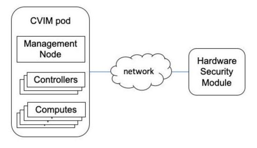
When Barbican is installed on a Cisco VIM pod, Cinder and Nova uses Barbican to store and retrieve volume encryption keys. Barbican is an optional service that can be included in the initial installation or added with a reconfigure operation. For details on how to enable Barbican see Enabling Barbican
