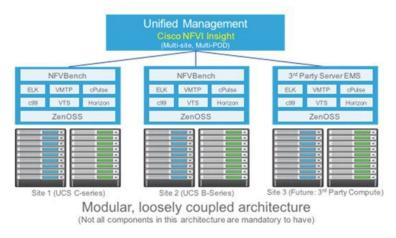
You can install UM on a standalone (BOM same as the management node) dedicated node to manage one or more Cisco VIM pods. As the UI interacts with the REST API, it is not necessary that the pod must be managed by UM node from Day 0. The UI interacts with each pod through REST API and Role Based Access Control (RBAC) information stored in the DB.
