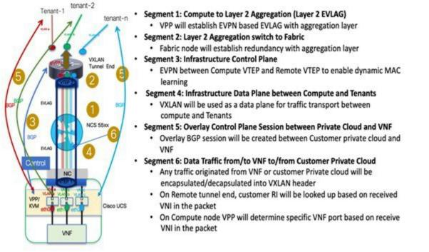
To set up Cisco VIM tenant L2 connectivity architecture, the following assumptions are made:
