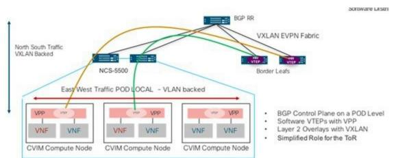
From a control plane point of view, three instances of GoBGP (in Active-Active Active mode) run on the controller nodes to establish L3 peering with the external BGP RR for importing or exporting VxLAN routes into or from Cisco VIM respectively. The imported information is then pushed into etcd, to maintain a single source of the information within Cisco VIM.
