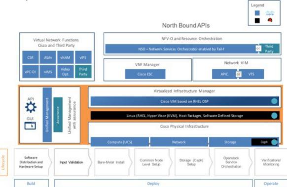
The following illustration shows a detailed view of the Cisco NFVI architecture and the Cisco NFVI installation flow
