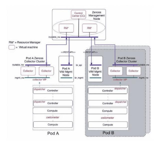
The NFVIMON architecture supports the monitoring of one or more Cisco VIM pods. There is no limit on the number of pods, but note that the setup supports up to ~ 25000 managed resources across pods, where a managed resource is a physical device, network device or virtual machine tracked from a monitoring perspective.
