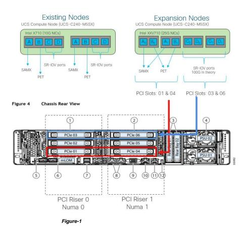
If user want to pick different configuration shown in *Figure-2* they have to update "setup\_data.yaml" as follow: hardware\_info: {NIC\_LEVEL\_REDUNDANCY: true, cpdp\_nic\_slot: [1,4], sriov\_nic\_slot: [2,5]} Here we are asking installer to pick PCIe 1 and PCIe 4 for CPDP ports and PCIe 2 and PCIe 5 for SRIOV ports.
