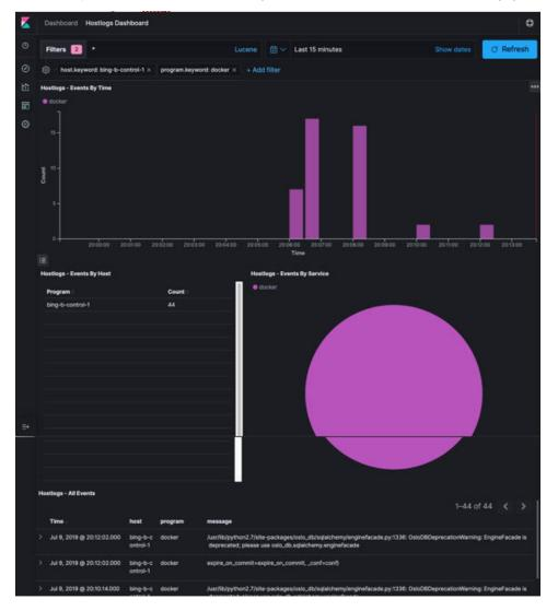
To know the log events in the Openstack for a given VM, enter the Lucene query (service: nova or service: neutron and message:<uuid>) in the Fi Iters field which is on top of the Dashboard. where <uuid> is obtained from Horizon website or by executing openstack nova list for the identifier of the instance. The following figure shows the Search Query page.
