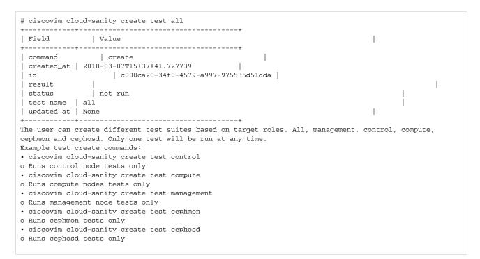
The cloud-sanity tests use the disk-maintenance and osd-maintenance tools, to assess overall health and status of the RAID disks and OSD status.
