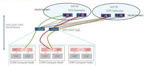
One set of VXLAN overlays manage the Cloud exchange traffic, while the other set of VXLAN overlays manage the Cloud management traffic. The multi-VXLAN (multi refers to 2) is used to conserve the number of bridge domains (BD) consumed on the Cisco NCS 5500 ToR.
