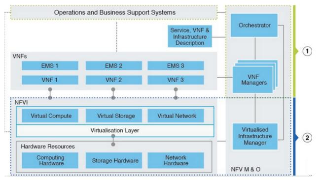
At a high level, the NFVI architecture includes a VNF Manager and NFV Infrastructure.
