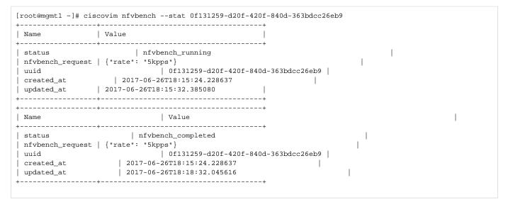
When the test is done, retrieve results in a JSON format:
