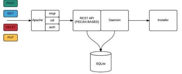
The Cisco VIM REST API security is provided by the Secure Sockets Layer (SSL) on the Apache web server. The *mod\_wsgi* running on the Rest API server calls the Pecan-based web application. The Pecan REST API server requires a username and password to authorize the REST API server requests.
