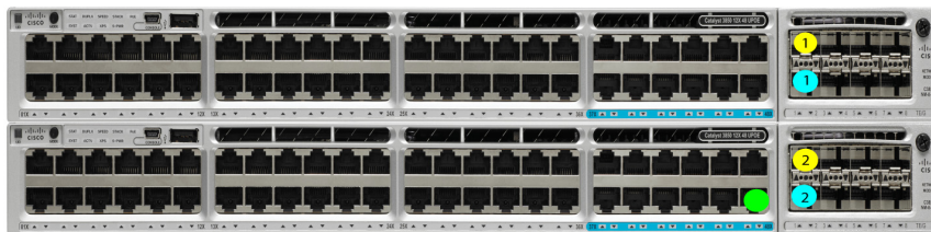
Dual 10/25GE ToR Switches (standalone or stacked)
