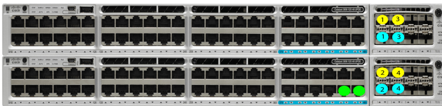
Dual 10/25GE ToR Switches (standalone or stacked)
