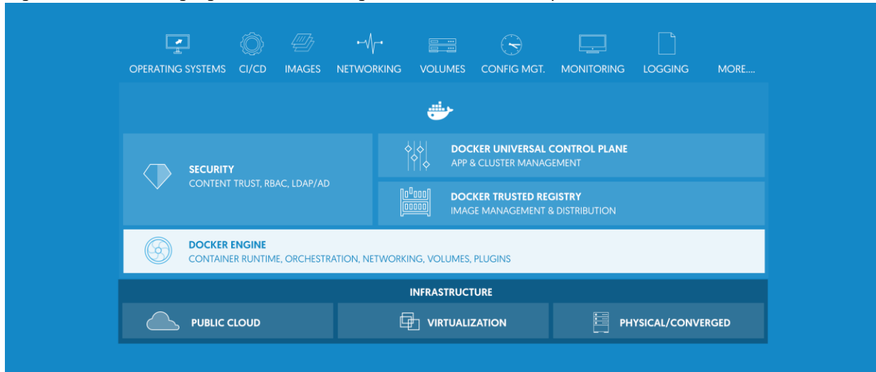
Figure 4 Following figure illustrates high-level Docker Enterprise Edition architecture
