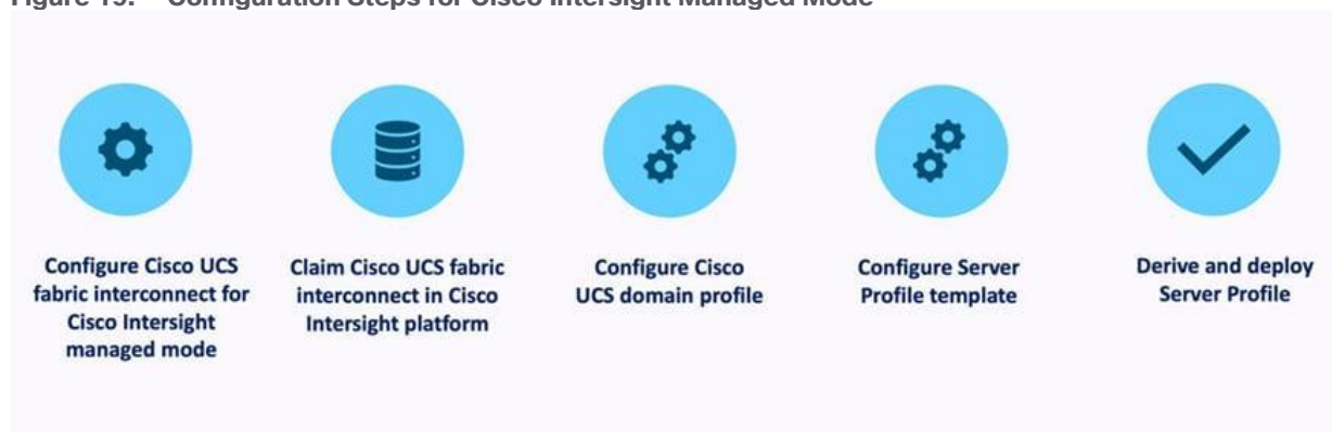
Figure 19. Configuration Steps for Cisco Intersight Managed Mode
