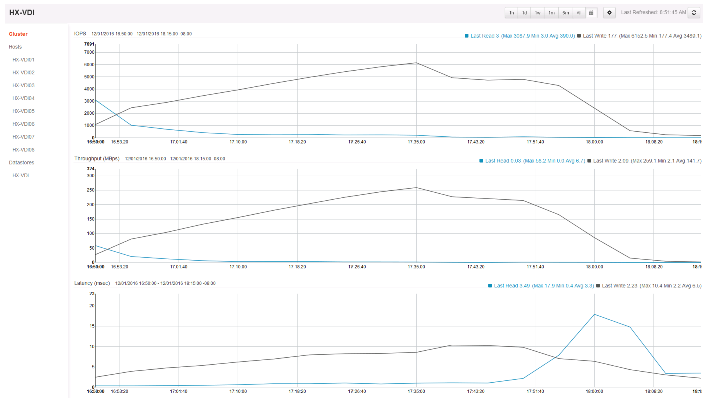
Figure 48 HyperFlex Cluster WebUI Performance Chart for Knowledge Worker Workload Running 1200 User Test on RDSH Server Windows Server 2012 R2
