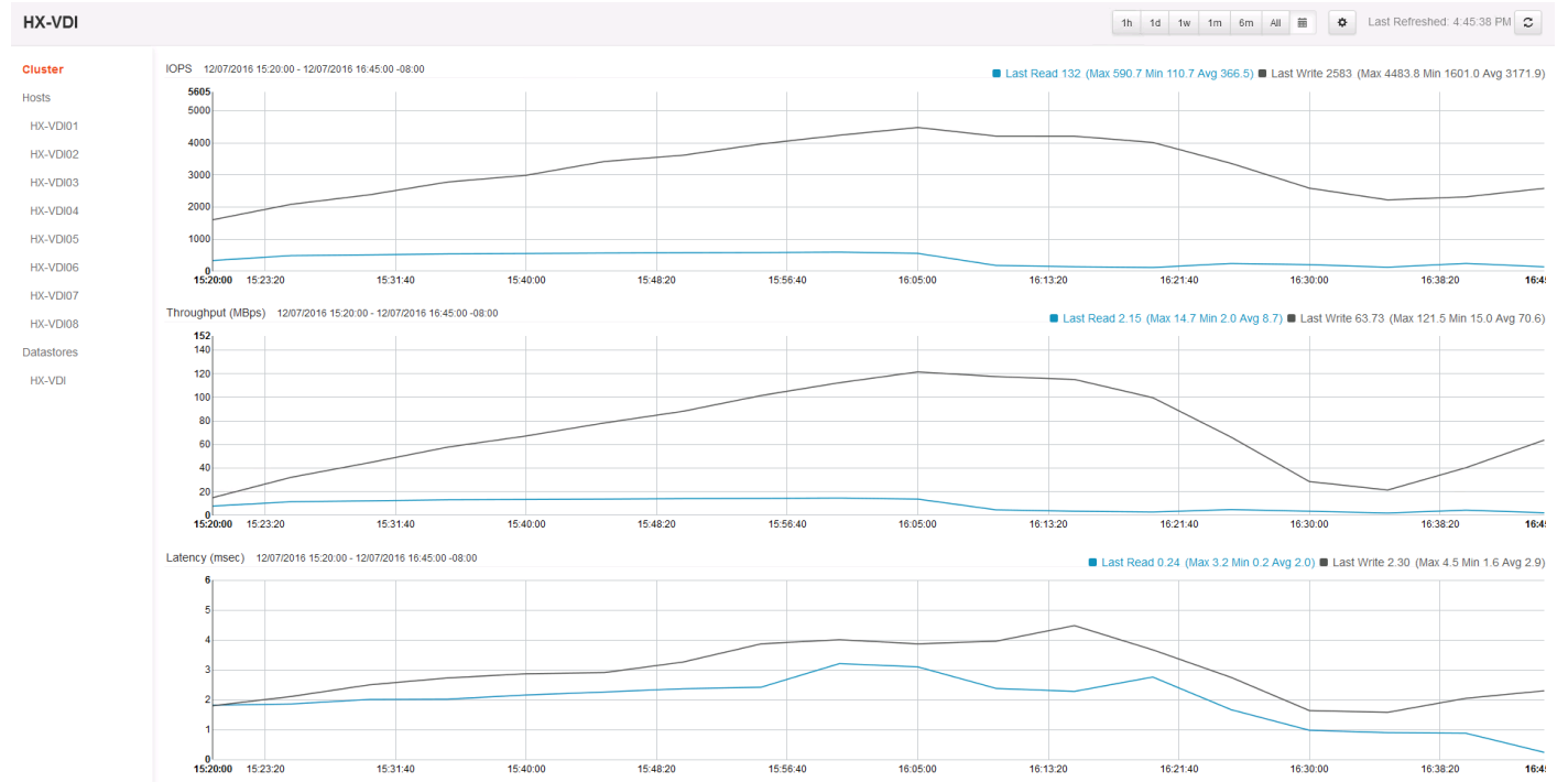
Figure 63 HyperFlex Cluster WebUI Performance Chart for Knowledge Worker Workload Running 750 User Test on Full Clone Windows 10 Virtual Desktops
