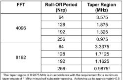
The taper region of 0.88/5 MHz is in accordance with the requirement for a minimum taper region of 1 MHz minus half subcarrier spacing. Achieving up to approximately 0.5 dB impact to the noise power in the adjacent spurious emissions integration region would allow a taper region of 0.8625 MHz, if the specification did not mandate the minimum taper region to be larger than this.
